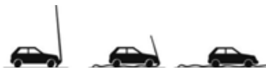
Figure 7. An example of the behavior of a pillar when a vehicle hits
