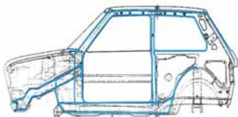
Figure 10. Places of application of structural adhesives on the body of a Koral vehicle
