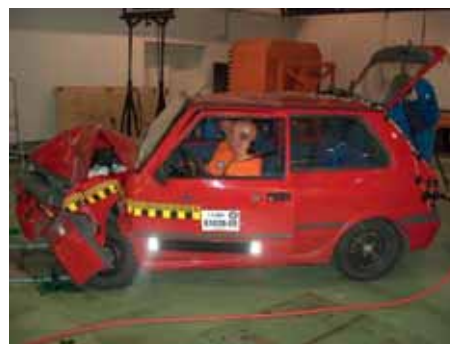
Figure 13. Vehicle after ECE test 94
