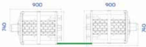
Figure 9. Dimensions SMA Tree (mm)
