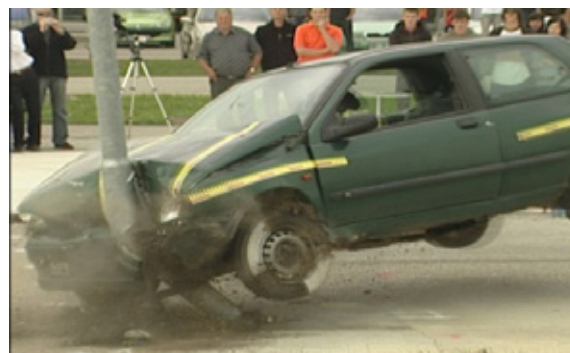
Figure 2. Vehicle stopping with an impact speed of 46 km/h, impact duration 0.5 seconds, deceleration 138 m/s 2
